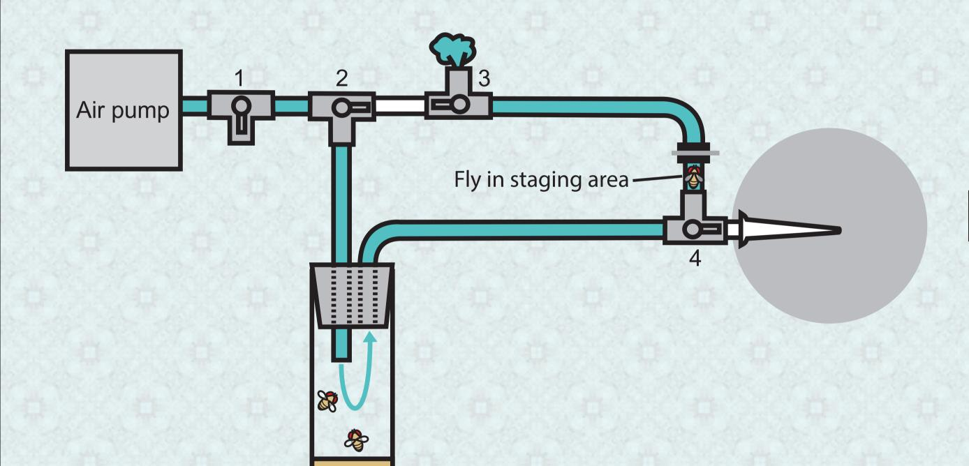
Airflow is directed through the fly vial, where a fly is picked up by the air stream and directed into the staging area.
